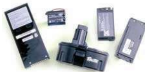
Common types of lithium-ion batteries
